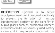
**PROPERTIES:** Thanks to micro glass balls with insulation features, it forms an insulating film to process a double-glazing effect (glass/air/glass) on the surfaces it is applied. With its 3.5 times lower thermal transmittance compared to other paints, it prevents the condensation of water vapor on the paint film, thus helping the prevention of heat
